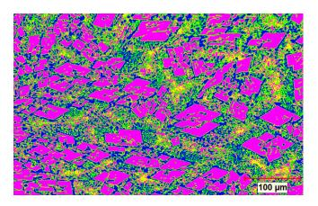
**Remarks:** Microstructure consists of Primary Metal Borides and Secondary Carbides in the matrix of Austenite & Martensite.
