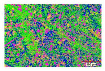
Remark: Microstructure shows primary chromium carbide and eutectic carbides along with austenite and martensite.
