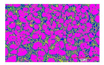
**Remarks:** Microstructure shows the Primary Chromium Carbides and Eutectic Carbides along with Austenite and Martensite
